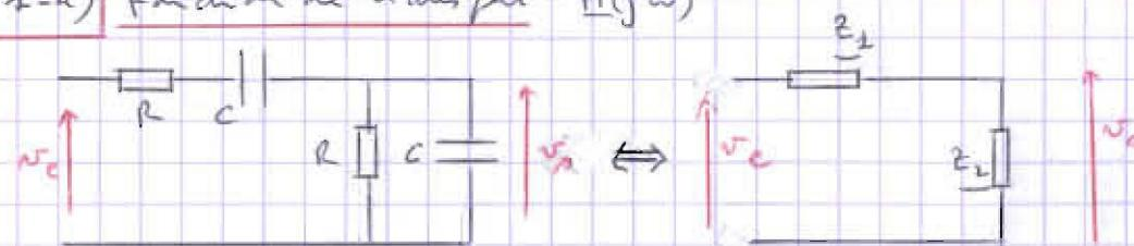
$$\text{Division de tension}, \frac{v_o}{v_e} = \frac{\underline{Z}_2}{\underline{Z}_1 + \underline{Z}_2} \frac{v_e}{v_e}$$
