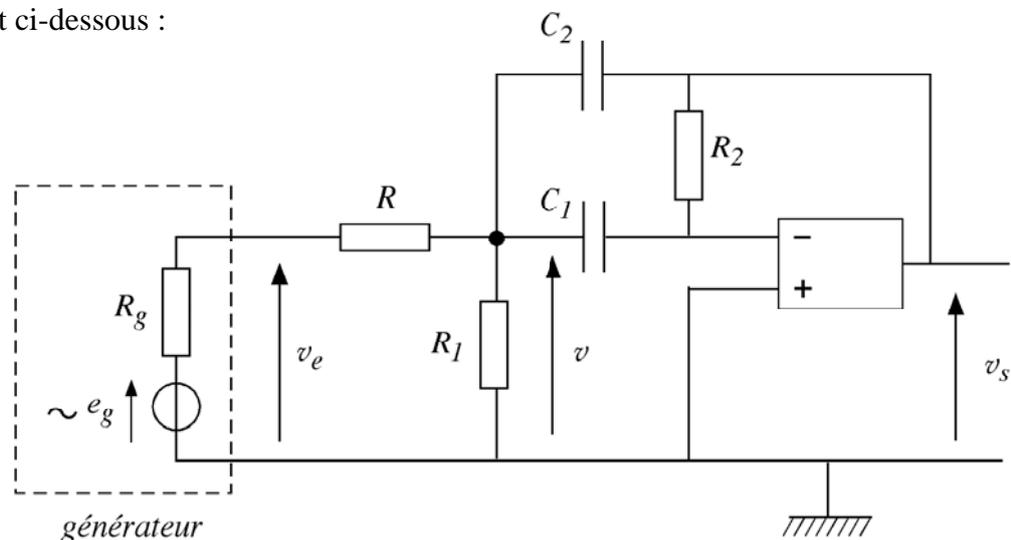
$$R = R_1 = R_2 = 100 \text{ k}\Omega \quad C_1 = C_2 = 2,2 \text{ nF}$$
